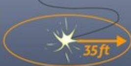
Downed power lines can energize the ground up to **35 feet away**. Even more in wet conditions.
